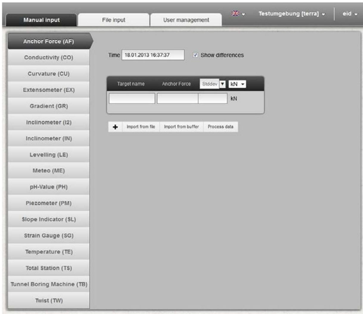
Figure 5. tManual Screenshot Showing a Sensor Array Ready for Online Manual Data Input
