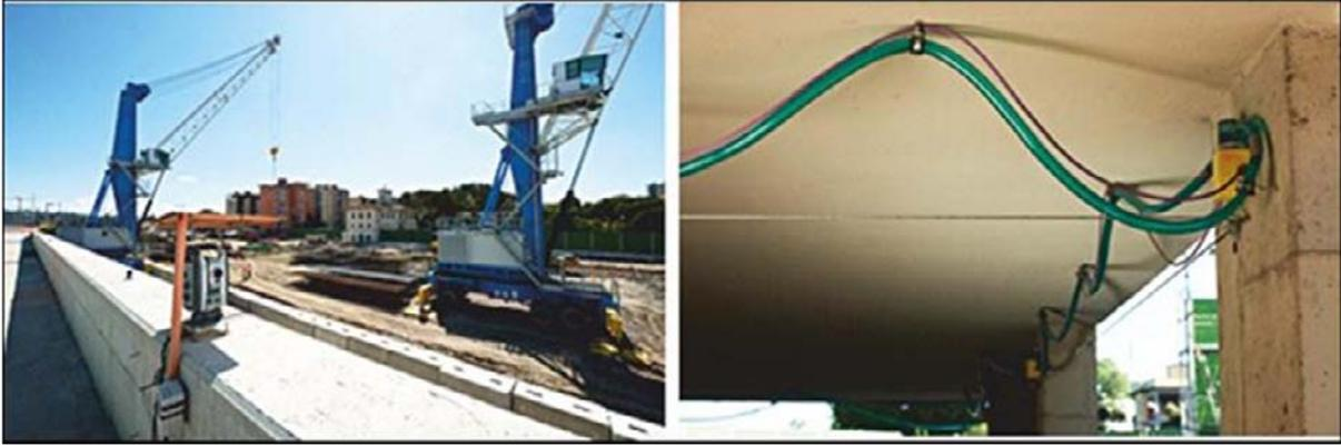
**Figure 4. Total Stations and Hydrostatic Levelling Systems at the Belfiore Site**
