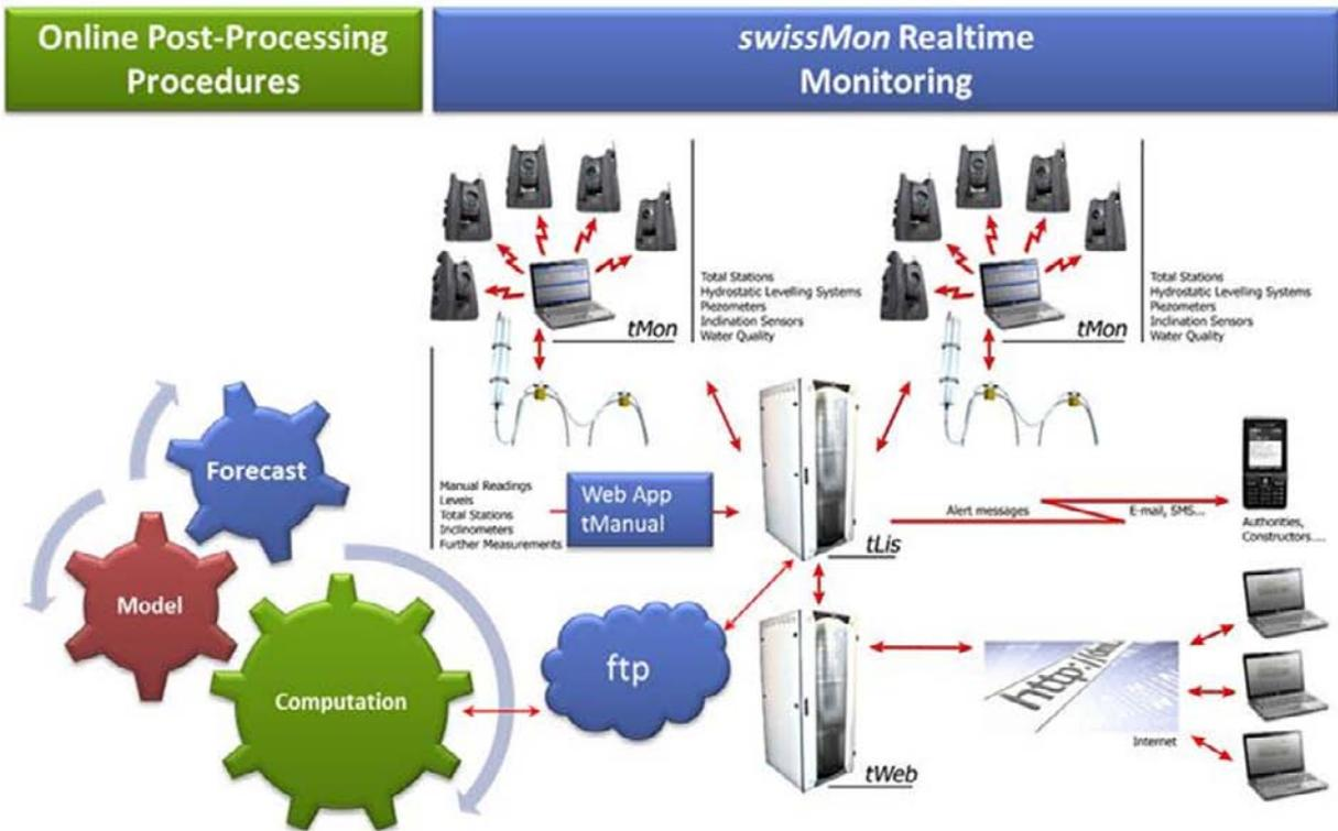
**Figure 6. Enhanced swissMon Architecture Specifically Developed for the “Nodo di Firenze” Project**
