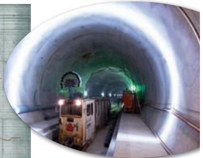
Figure 1: tunnel locomotive with cameras and lighting
